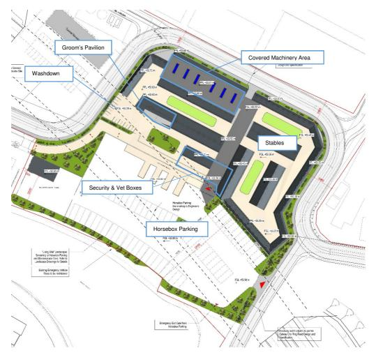
Figure 4 – Proposed Permanent Stableyard Site Layout
